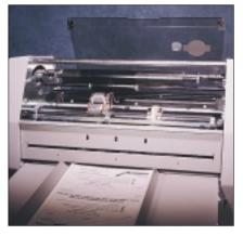
An optional re-inking system enables you to use Pantone inks. The system produces thousands of impression before it needs re-inking.
