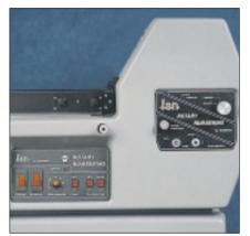
Controls are centrally located for ease of operation. Both the FRN 5 and FSN have platen pressure adjustment. The numbering position can also be adjusted whilst the machine is in operation.
