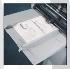
A sophisticated sensing system controls the numbering action. Several numbering heads can be fitted and both convex and parallel heads can be run, simultaneously.
