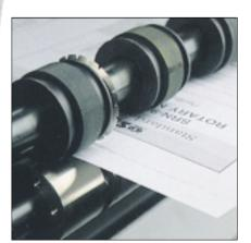
Slitting perforators give flat perforating on a wide range of stocks. Various perforating, slitting and scoring wheels are available.
